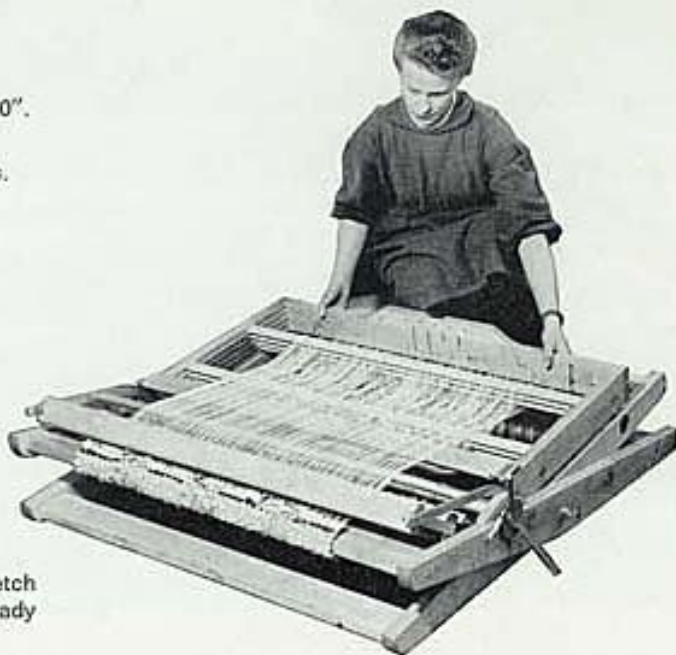
FL-4 40" FLOOR LOOM COLLAPSED
